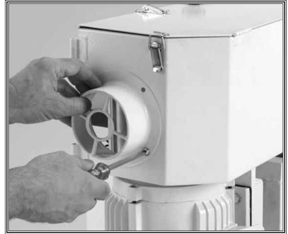
Figure 14. Dust port installation.
