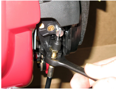
Figure 12: Throttle cable adjustment
