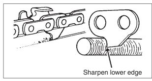
Important points for proper maintenance of saw chain:
