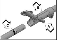
Note: Lower bearing housing and head assembly must be in line with the engine.
