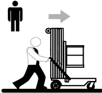
Figure 1-6. Use Handles Provided On Mast Crossbar To Move Machine.
