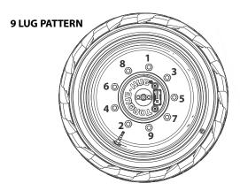
**3.** The tightening of the nuts should be done in stages. Using the recommended sequence, tighten the nuts per wheel torque chart following.
