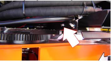
Lube Point(s) - 1 Grease Fittings Capacity - A/R
