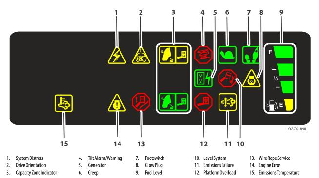
**Figure 3-9. Platform Control Indicator Panel**
