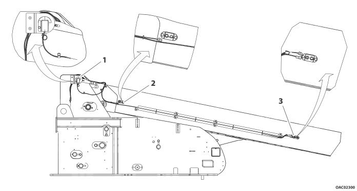
Figure 2-2. Horizontal and Capacity Proximity Sensors- Sheet 1 of 2
