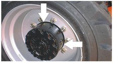
Lube Point(s) - Level/Fill Plug Capacity - 44 oz. (1.3 L) - 1/2 Full Lube - EPGL
