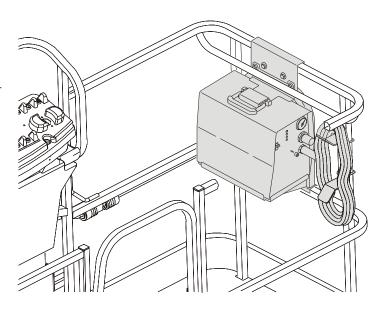
SkyCutter™ is capable of cutting up to a thickness of 3/8" metal. It can produce 27 A at 92 VDC at 35% duty cycle or 14 A at 92 VDC at 60% duty cycle. It receives power from the SkyPower™ system.
