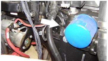
Lube Point(s) - Fill Cap/Spin-on Element
