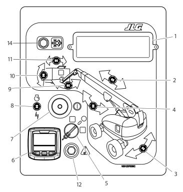
Figure 3-6. Ground Control Console - 860SJ with MSSO and DPF
