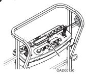
Cable is pressed, breaking the magnetic connection between the cable and right bracket.
