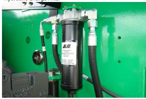
Interval - Change after first 50 hours and every 6 months or 300 hours thereafter or as indicated by Condition Indicator (if equipped).
