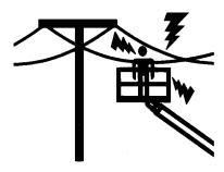
It is not recommended to use the machine during lightning. To prevent injury or machine damage if lightning occurs during operation, lower the boom and shut down the machine in a safe and secure location.
