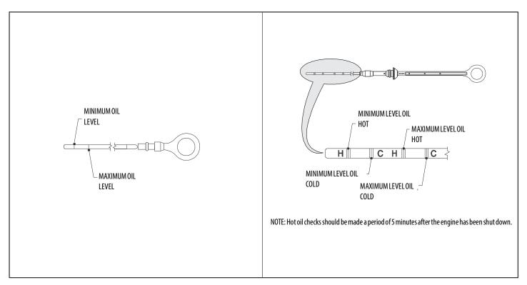
Figure 7-5. Deutz 2011 Engine Dipstick
