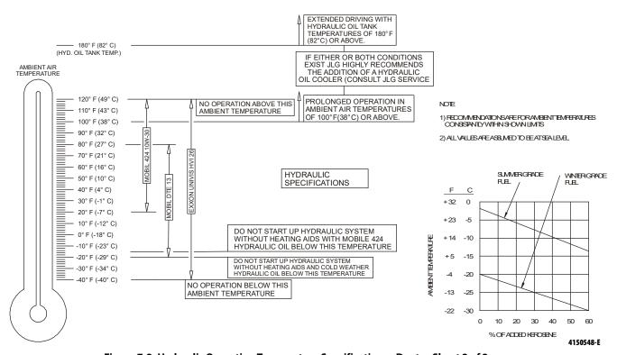
Figure 7-3. Hydraulic Operating Temperature Specifications - Deutz - Sheet 2 of 2
