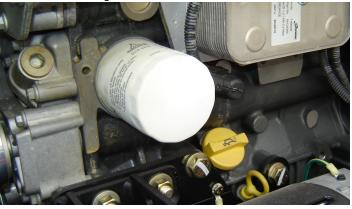
Lube Point(s) - Fill Cap/Spin-on Element
