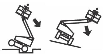
Do not elevate platform or drive with platform elevated while on or near a sloping, uneven, or soft surface. Ensure machine is positioned on a smooth, firm surface within the limits of the maximum operating slope before elevating platform or driving with the platform in the elevated position.
