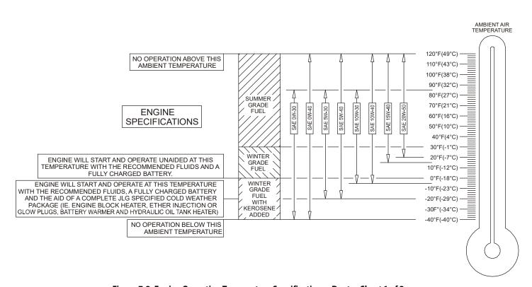
Figure 7-2. Engine Operating Temperature Specifications - Deutz - Sheet 1 of 2
