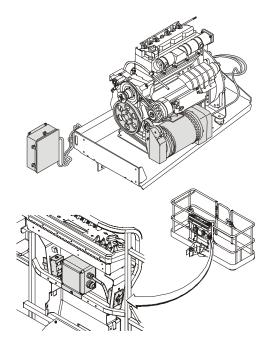
The SkyPower™ and generator systems supply AC power to the platform through an AC receptacle to run tools, lights, cutting, and welding equipment.
