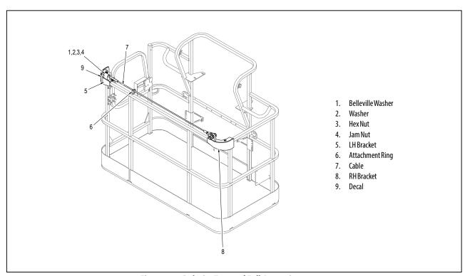
Figure 6-2. Bolt-On External Fall Arrest System
