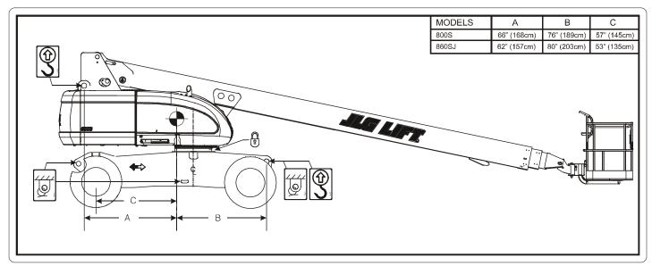
Figure 4-7. Lifting and Tie Down Chart
