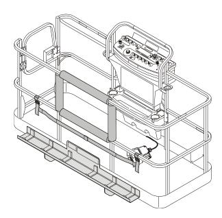
SkyGlazier™ allows glaziers to position panels efficiently. The glazier package consists of a tray that attaches the bottom of the platform. The panel rests on the tray and against top-rail of the platform, which is padded to prevent damage. SkyGlazier™ includes a strap to secure the panel to the platform rail.
