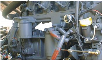
Lube Point(s) - Fill Cap/Spin-on Element
