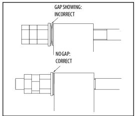
Figure 6-1. Bolt-On External Fall Arrest Cable
