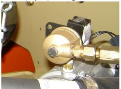
Interval - 3 Months or 150 hours of operation Comments - Replace filter. Refer to Section 7.7, Propane Fuel Filter Replacement
