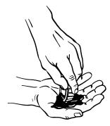
Lube Point(s) - Repack Capacity - A/R Lube - MPG Interval - Every 2 years or 1200 hours of operation 3. Swing Drive Hub
