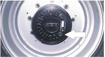
Lube Point(s) - Level/Fill Plug Capacity - 20 oz. (0.6 L) Lube - EPGL Interval - Check level every 3 months or 150 hrs of operation; change every 2 years or 1200 hours of operation 5. Hydraulic Return Filter
