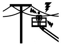
• It is not recommended to use the machine during lightning. To prevent injury or machine damage if lightning occurs during operation, lower the boom and shut down the machine in a safe and secure location.
