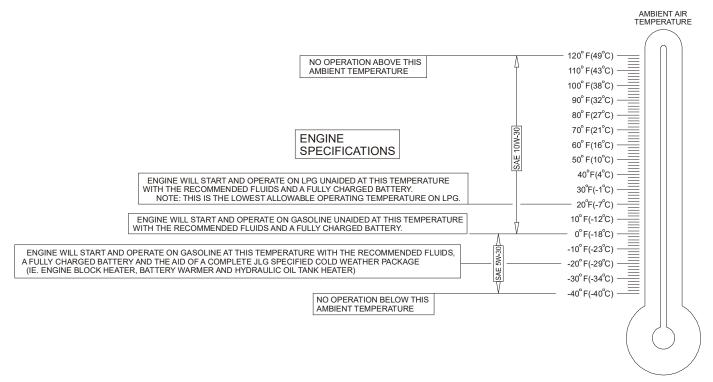
Figure 7-3. Hydraulic System Operating Temperature Specifications - Sheet 1 of 2
