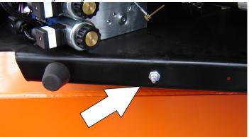
Lube Point(s) - 1 Grease Fittings Capacity - A/R Lube - MPG Interval - Every 3 months or 150 hrs of operation Comments - Remote Access. Apply grease and rotate in 90 degree intervals until bearing is completely lubricated. 2. Wheel Bearings (If equipped)
