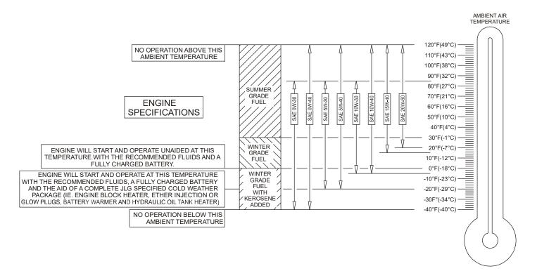
Figure 7-1. Engine Operating Temperature Specifications - Deutz - Sheet 1 of 2
