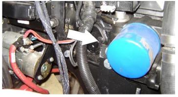
Lube Point(s) - Fill Cap/Spin-on Element Capacity - 4.5 qt. (4.25 L) w/filter Lube - EO Interval - 3 Months or 150 hours of operation Comments - Check level daily/Change in accordance with engine manual. 10. A. Fuel Filter - Deutz
