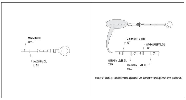
Figure 7-5. Deutz 2011 Engine Dipstick
