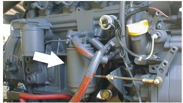
On Engine: Lube Point(s) - Replaceable Element Interval - Change in accordance with engine manual
