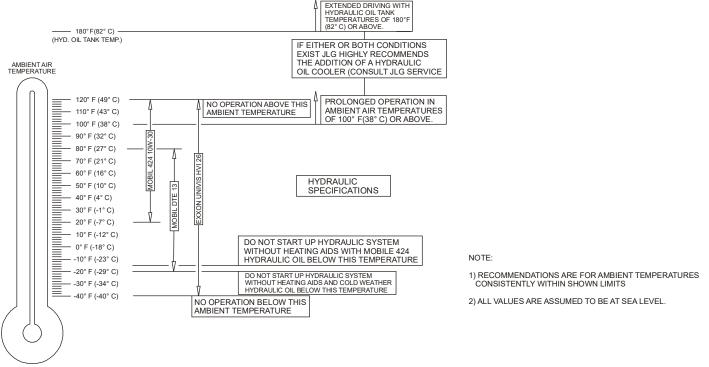
Figure 7-4. Hydraulic System Operating Temperature Specifications - Sheet 2 of 2 4150548-E
