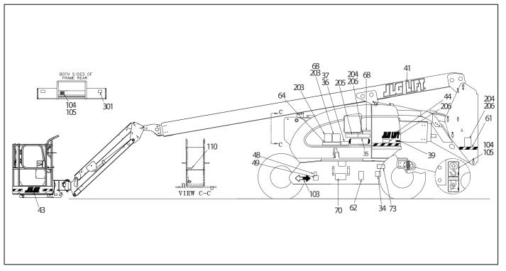
Figure 4-8. 600AJ Decal Installation - Sheet 1 of 4
