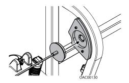
Reattach magnetic end of cable to bracket if it becomes disconnected.
