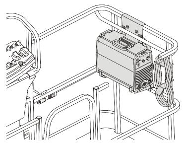
SkyWelder<sup>™</sup> is capable of TIG and Stick welding, producing 200 Amps at 100% duty cycle or 250 Amps at 50% duty cycle. This accessory receives power from the SkyPower<sup>™</sup> system.
