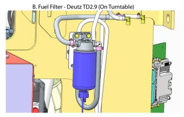
Lube Point(s) - Replaceable Element Interval - Change in accordance with engine manual
