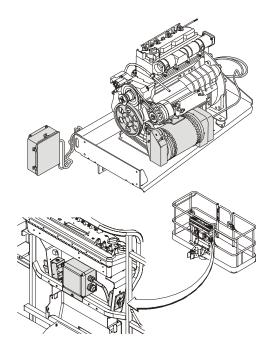
The SkyPower<sup>™</sup> and generator systems supply AC power to the platform through an AC receptacle to run tools, lights, cutting, and welding equipment.
