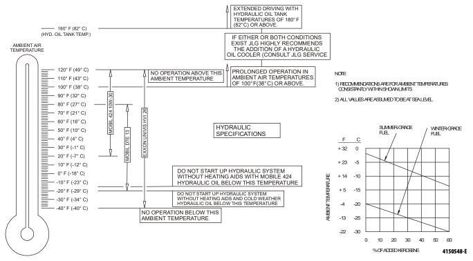
Figure 7-2. Hydraulic Operating Temperature Specifications - Deutz - Sheet 2 of 2
