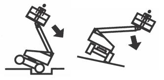
• Do not elevate platform or drive with platform elevated while on or near a sloping, uneven, or soft surface. Ensure machine is positioned on a smooth, firm surface within the limits of the maximum operating slope before elevating platform or driving with the platform in the elevated position.
