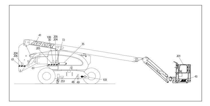
Figure 4-9. 600AJ Decal Installation - Sheet 2 of 4
