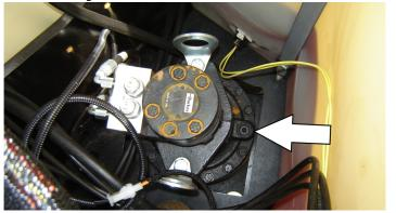
Lube Point(s) - Level/Fill Plug Capacity - 43 oz. (1.3 L) Lube - 90w80 Gear Oil Interval - Check level every 3 months or 150 hrs of operation; change every 2 years or 1200 hours of operation
