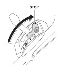
When the mower is not in use, turn the fuel valve to the OFF position.
