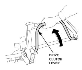
While holding the drive clutch lever all the way forward, look through the cover plate hole and check the position of the control arm.
