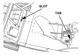
Make sure the tab at the bottom rear of the mulching plug fits snugly into the slot at the back of the discharge chute.
