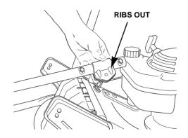
Insert the 8 x 40 mm lower handle bolts and finger tighten them.
