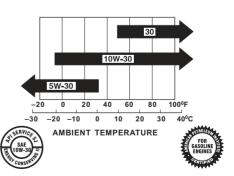
The SAE oil viscosity and service classification are in the API label on the oil container. Honda recommends API SERVICE category SJ or later oil with the ILSAC "starburst" certification mark displayed on the container.
