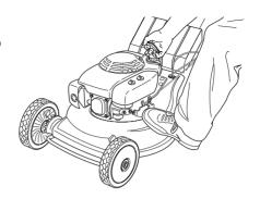
4. If the CHOKE position was used during starting, move the throttle lever away from the CHOKE position as soon as the engine warms up enough to run smoothly without use of the choke. Set the throttle lever at FAST to mow or at SLOW to idle.
