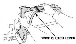
You can control self-propelled speed with the drive clutch lever. The mower will move gradually faster as you push the drive clutch lever forward. If you push the lever all the way forward to the handlebar, the mower will move at the speed determined by the shift lever setting (page 21).
