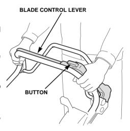
This will help to prevent stalling the engine, and it will also extend the service life of the blade control mechanism.
