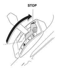
Turn the fuel valve to the OFF position. This will prevent carburetor flooding and reduce the possibility of fuel leakage.
