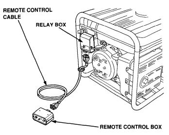
NOTE: • Connect the blind connector when not using the remote control.
