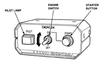
Starting the engine with remote control
