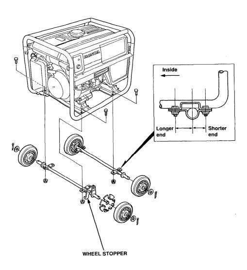
NOTE: Install the shaft with wheel stopper facing engine side.
