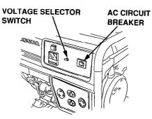
Do not exceed the current limit specified for any one receptacle. If an overloaded circuit causes the AC circuit breaker or circuit protector to switch OFF, reduce the electrical load on the circuit, wait a few minutes and then reset the circuit breaker.
