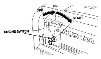
Return the key to the ON position once the engine has started. Do not use the starter for more than 5 seconds at a time. If the engine fails to start, release the switch and wait 10 seconds before operating the starter again.
