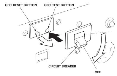
6. Press the GFCI RESET button. The RESET button should stay in, flush with its base plate.
