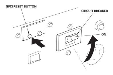
During generator use, if the GFCI RESET button extends and the circuit breaker trips, this usually indicates a faulty power tool, appliance, or cord.
