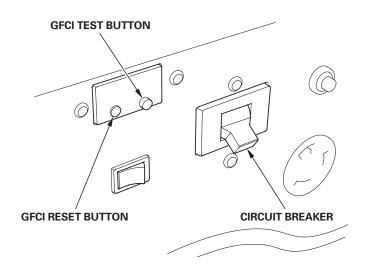
Observe the following precautions to ensure proper GFCI operation and to reduce shock hazards:
