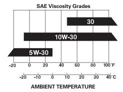
SAE 10W-30 is recommended for general, all-temperature use. Other viscosities shown in the chart may be used when the average temperature in your area is within the indicated range.
