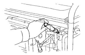
7. After the spark plug is seated, tighten with a spark plug wrench to compress the washer.
