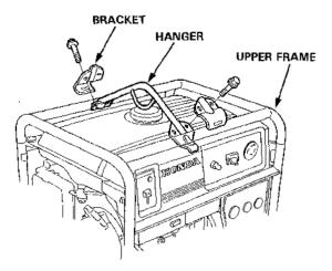
NOTE: Install at near center avoiding to install over the fuel filler cap.
