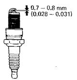
6. Check that the spark plug washer is in good condition, and thread the spark plug in by hand to prevent cross-threading.
