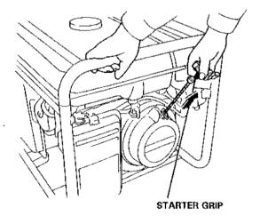
7. Push the choke rod to the OPEN position as the Engine warms up.
