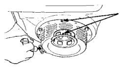
Align the notch on the starter pulley with the hole at the top of recoil starter.
