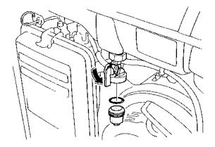
d. Drain the carburetor by loosening the drain screw. Drain the gasoline into a suitable container.
