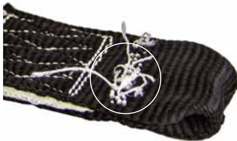
Broken/damaged indicator stitching - Immediately remove from service!
