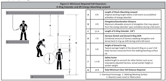
NOTE: Use of an extender will increase the users potential fall distance. The user must be sure the increased total length of a lanyard is accounted for in calculating fall clearance distances, including swing fall. Be aware that when using an SRL, there may be additional fall clearance required depending on anchor point location. If unsure, consult a Competent Person.
