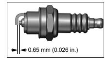
2. Correct the spark gap if it is wider or narrower than the standard gap.
