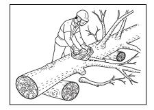
Don't cut with the saw overhead or aligned vertically with your body. If the saw should kickback, you may not have enough control to prevent possible injury.
