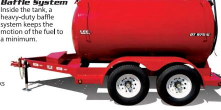
Unlike square tanks, round tanks distribute the stress of surging diesel evenly around the tank.
