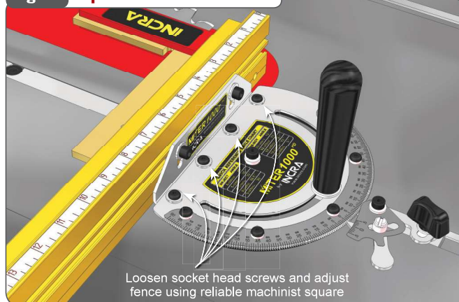
Fig. 8 Square Fence to Blade
