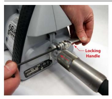
Figure 8: Locking lever adjustment
