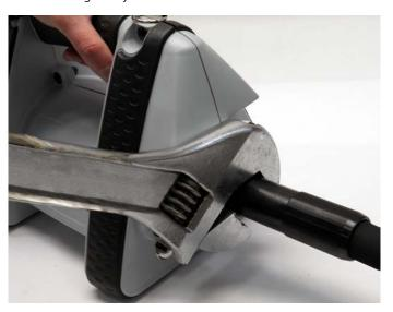
Figure 12: Hex motor connection
