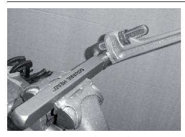
Figure 14: End cap removal
