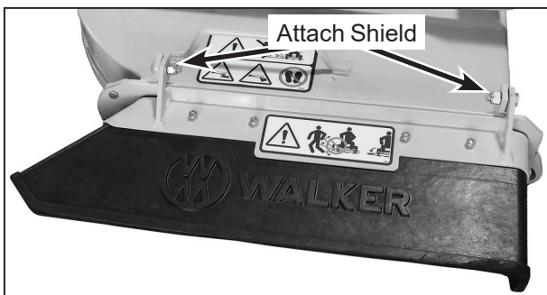
Discharge Shield Installation on Side Discharge Deck
