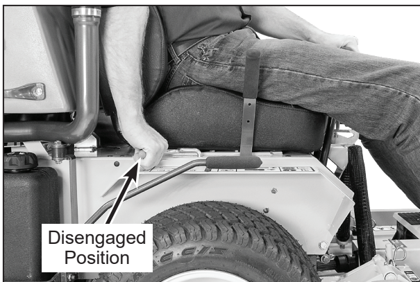
Parking Brake Disengaged
