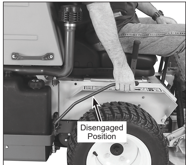
Blade Clutch Disengaged
