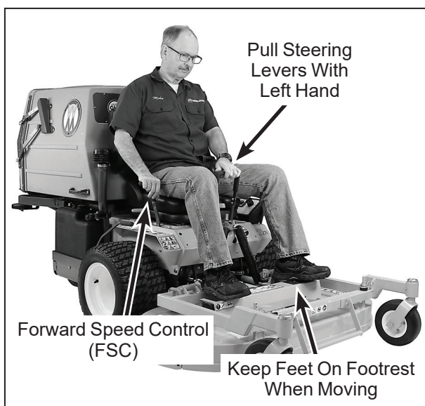
Correct Operator Hand Position on the Controls
