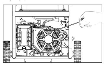
5. Do not over-choke. As soon as engine starts, move the choke lever to the "RUN" position over a 2-5 second duration.
