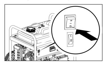
4. *If generator was started electrically,* press the battery switch to the "OFF" position.
