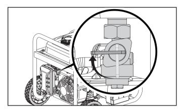
**Important:** Always ensure that the fuel valve, the ignition switch, and the battery switch are in the "OFF" position when the generator will not be used for an extended period of time.
