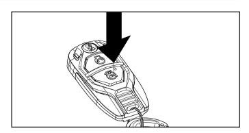
5. Push and release the START **b** button on the remote key fob. The red light blinks once to program the remote.
