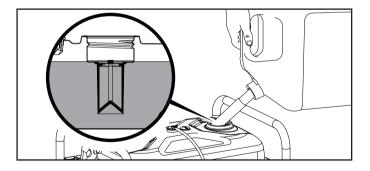
3. The approximate fuel level is shown on the fuel gauge on top of the fuel tank.
