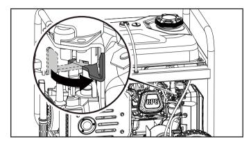
3. Push the ignition switch to the "ON" position.
