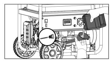
4. Check engine oil level at every use and add as needed.
