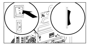
2. Turn the battery switch to the "ON" position.
