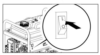
Press and hold the ignition switch to the "START" position. Release as the engine begins to start. If the engine fails to start within five seconds, release the switch and wait at least ten seconds before attempting to start the engine again.
