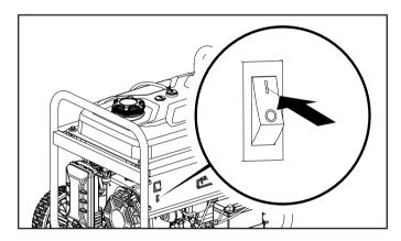
2. Push the ignition switch to the "ON" position.
