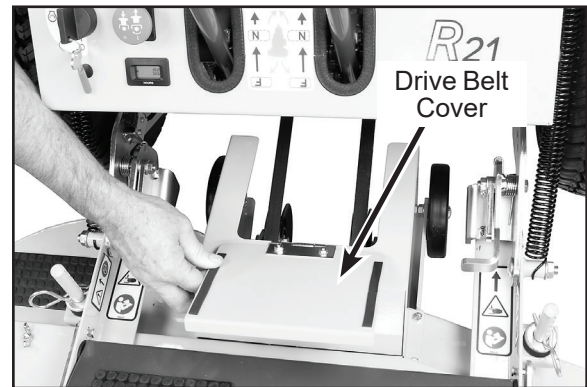
Lift Drive Belt Cover to Route the Belt
