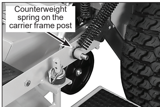
Counterweight Spring on Carrier Frame
