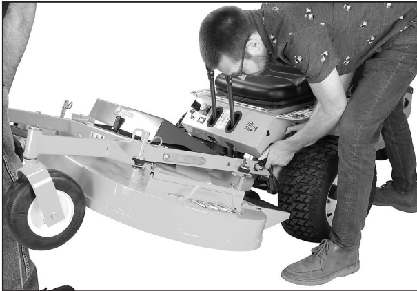
Install Counterweight Spring on Carrier Frame
