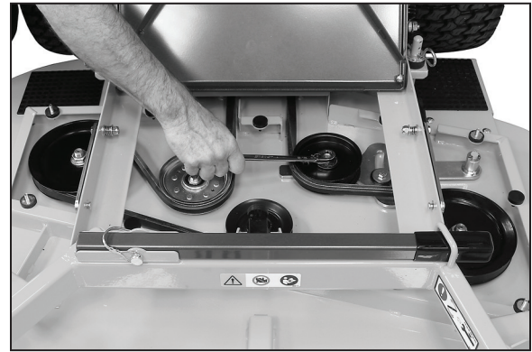
Tension Belt with Deck Idler Arm
