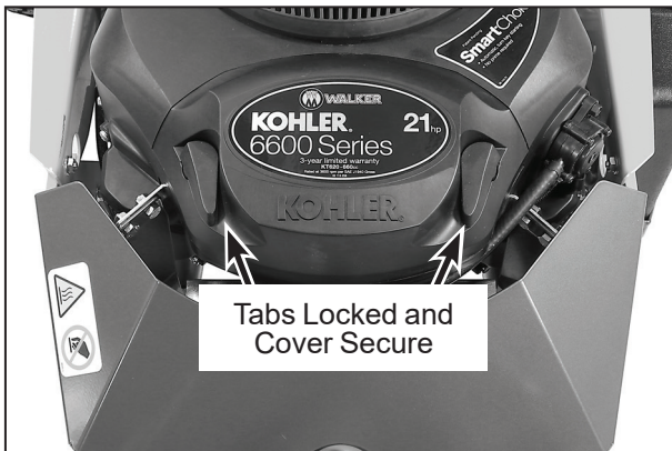
Air Filtration Installed
