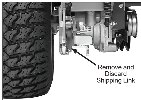
Shipping Link on RH Deck Support Arm
