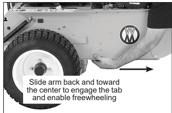
Engage Transaxle LOCKOUT (LH shown)
