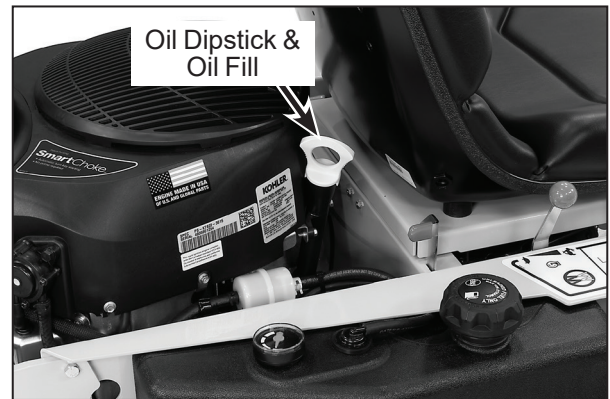
Oil Dipstick and Oil Fill Location
