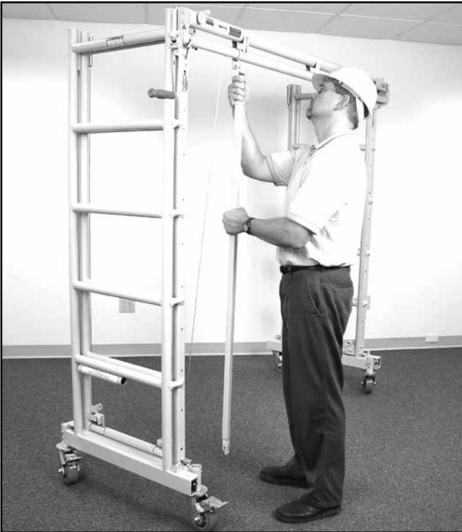
6) Attach braces between the beam and the base of each end section. WARNING: NEVER operate the Tele-Tower Adjustable Work Platform without these braces. Doing so can result in damage to the structure which can lead to failure that can result in severe property damage and or severe bodily injury or death.
