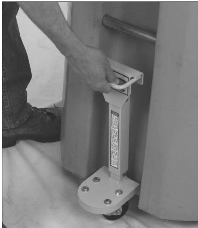
1) Place the lower hook of the Troll® EZ Wheel™ under the front edge of the container.
