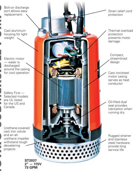
**Multiquip Electric Submersible Pumps** are ideal for removing water from confined areas. Their compact design and high performance enables them to get the job done where other pumps come up short.
