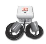
All MQ 115V 1Ø pumps are designed with internal thermal overload protection and do not require extra electrical protection, however, the **CB3 control box** is offered for convenient ON/OFF/AUTO and float switch operations. The CB3 comes with two SW1WOPA Float switches.
