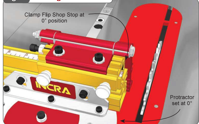
Fig. 13 Zeroing Fence Scale
