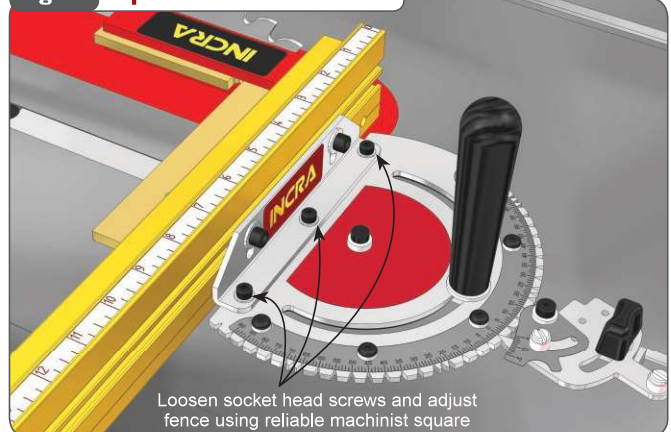
Fig. 8 Square Fence to Blade
