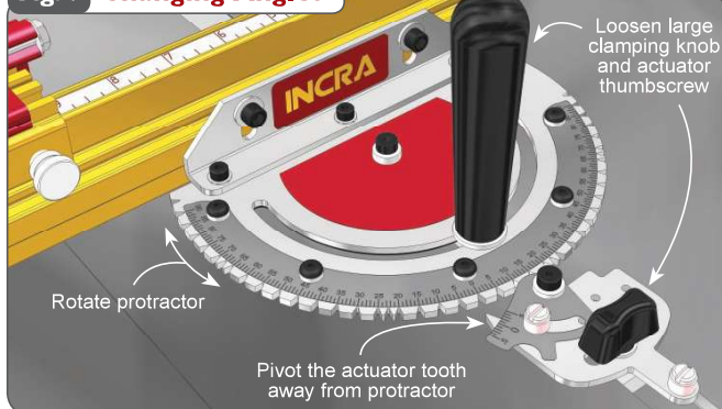
Fig. 10 Locking the Protractor
