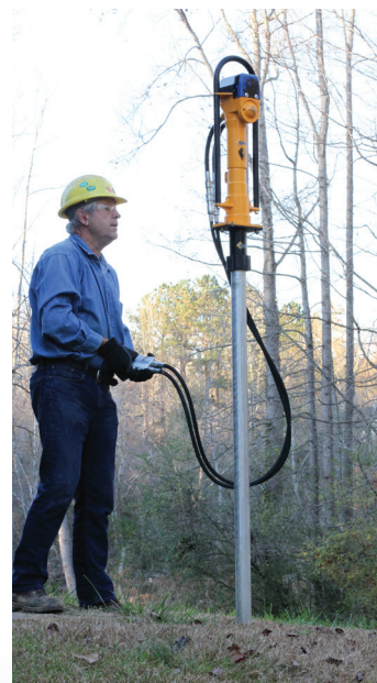
Use of optional remote valve (801011) with HPD 60.
