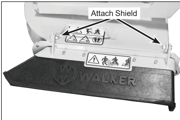
Deck Discharge Shield Installation
