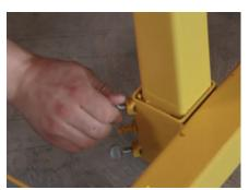
**2**. Tighten both lock screws on the dolly base to hold the boom tube securely.
