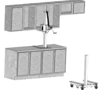
2. Use the Counter Base Configuration for final positioning of the cabinets.
