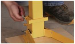
**2.** Tighten the thumb screws on the Counter Base to hold the Boom firmly in place. Install either of the boom sections into the Counter Base.
