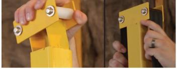
**7**. Insert the top roller assembly then position the strap over the top rollers, raising the Collar up the Boom.
