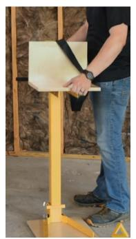
**3.** Let out a 2' loop of strap on the Collar Assembly and slide the Collar Assembly over the Boom Tube.
