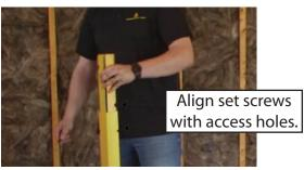
**4.** Insert the split boom connector. Align the set screws with the access holes in the boom tube.
