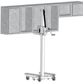
2. Operate the winch to raise cabinets into place. Lock the brakes on the casters and level the cabinets and fasten in place.
